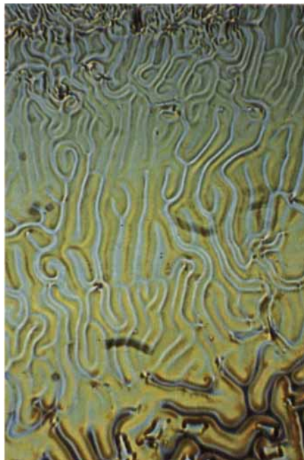
Figure 7. A contact preparation of 97 per cent (wt/wt) of compound 2 and 9O2Cl3MT showing the continuous chiral nematic phase at 108°C.
